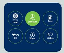
Driving with underinflated or overinflated tyres can adversely affect your braking distance, steering, fuel efficiency and lifetime of your tyres.
